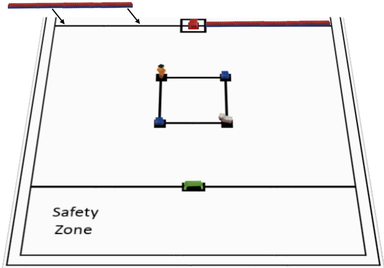
The four task objects (not the Fire block or barrier) will be set up, randomly, on one of the four corners of the task square, so that they are completely within the black squares. An example lay out is shown above.
