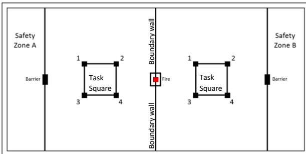
There is a 300mm deep Safety Zone at either end of the table, separated from the rest of the field by a black line. There is a small black rectangle (8mm x 4mm) on the black line. One robot will start in Safety Zone A and the other in Safety Zone B.
